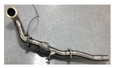
13 Note the orientation of the OE chassis bracket on the OE downpipe. Remove the OE chassis bracket from the newly-freed OE downpipe and install onto the Revo mid pipe in the same orientation
