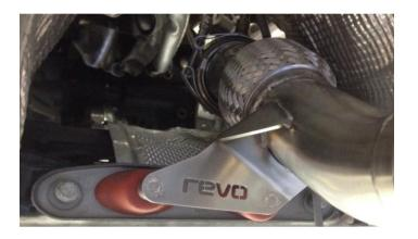
From the top of the vehicle, install the Revo test pipe or optional catalytic converter section onto the turbocharger exhaust housing flange using the OE V-band clamp. Pinch the clamp ears to seat the Revo flange onto the turbocharger and install the OE clamp bolt finger tight, ensuring that the Revo test/catalytic converter pipe can still rotate within the clamp
