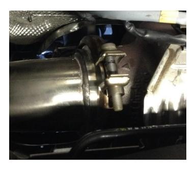
17 Install the OE slip fit clamp over both the Revo reducer and OE exhaust pipe to hold the reducer section of the Revo downpipe up. Tighten the clamp so that the Revo reducer section can still rotate within the clamp.
