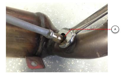
Using an oxygen sensor socket or 22mm wrench, assemble the OE oxygen sensor into either the optional Revo catalytic converter pipe or the Revo test pipe after applying anti-sieze to the threaded area of the sensor only. Install the oxygen sensor finger tight and tighten 1/4 turn (approx. 55 Nm [41 ft.-lbs.])
