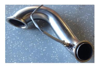
12 Using a 13mm deep-well socket, loosely assembly all (3) Revo pipes with the (2) provided V-band clamps in the configuration shown at right. Be sure that the pipes can still rotate within the clamps before continuing
