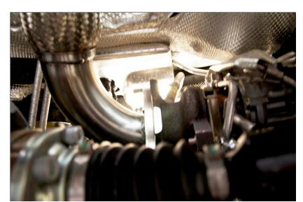
3. Install the downpipe onto the studs and **finger-tighten the nuts**.
