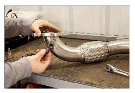
3. You'll start with the downpipe and work your way back. Install the downpipe onto the studs and **finger-tighten the nuts**.
