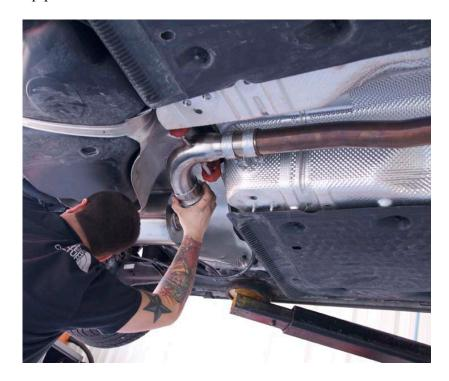
3. Install the rear muffler. Install into hangers first to make it easier to handle, then clamp it as in step 2. Verify alignment in bumper cutouts before the final torque.
