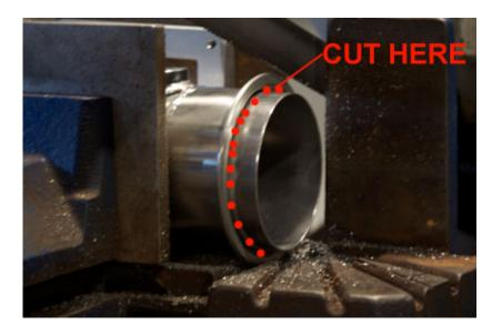
2. If necessary, grind to create a smooth surface.
