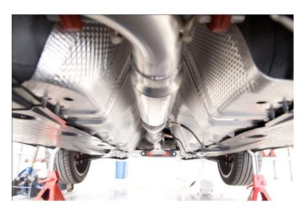
9. Install the first muffler section into the hanger, then clamp it with the J-pipe.
