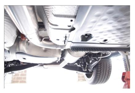
10. Install the rear muffler. Install into hangers first to make it easier to handle, then clamp it as in step 7. Verify alignment in bumper cutouts before the final torque.
