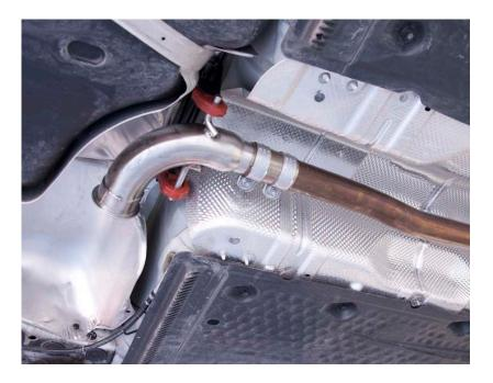
2. Install the first muffler section into the hanger, then clamp it with the J-pipe.
