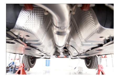
6. Install the first muffler section into the hanger, then clamp it with the J-pipe.
