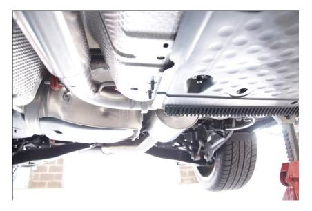
7. Install the rear muffler. Install into hangers first to make it easier to handle, then clamp it as in step 7. Verify alignment in bumper cutouts before the final torque.
