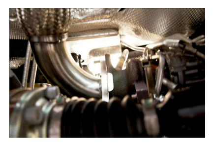
4. Using a supplied v-band clamp, install the catalytic midpipe section (optional) or test pipe section, angling the O2 sensors out of the way before tightening.
