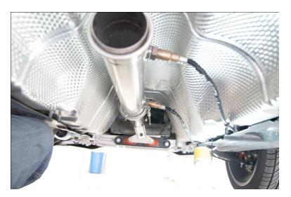
5. Install the J-pipe with a v-band clamp, leaving it slightly loose for now.
